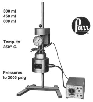
All of the safety and convenience features offered in larger PARR pressure reactors are included in these smaller units, making them well suited for a variety of chemical operations. They are available in all principal corrosion resistant alloys. For details, write or phone: Parr Instrument Company, Moline, Illinois 61265. 309/762-7716
